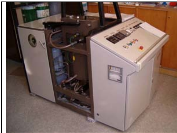
Figure 5. Hot Isostatic Pressing (HIP).
